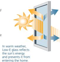
In cold weather, Low-E glass reduces the amount of heat lost by reflecting it back inside.
